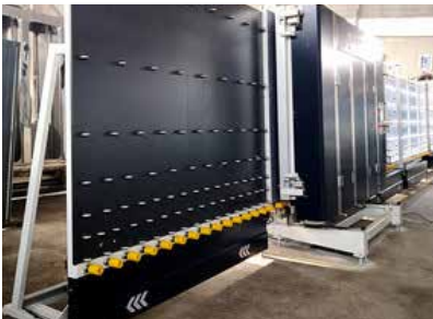
Double Glazing Line
